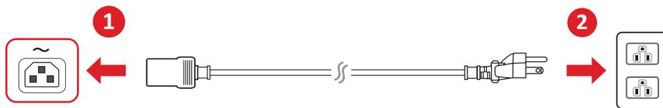
1. Connect the power cord to the AC IN jack at the rear of the monitor.
